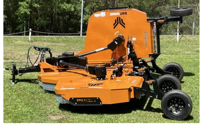
Smooth top prevents accumulation of debris. Fully baffled 4.55mm high-strength steel frame. 6.5mm thick and 330mm deep side skirt for maximum handling of cut material.
