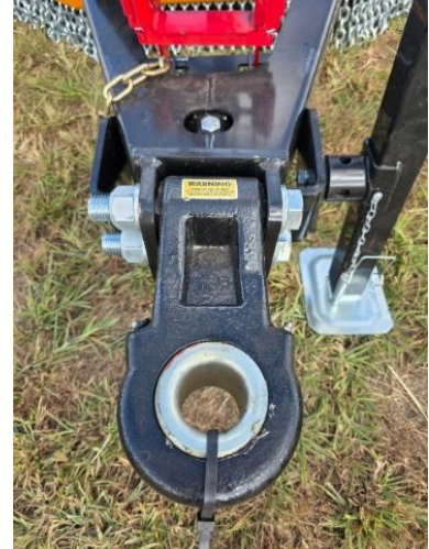
Heavy Duty Swivel towing eye reduces stress on equipment.
