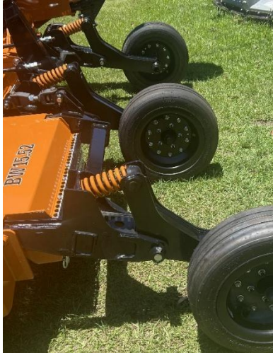
Individual axle sprung wheels ensuring even cut and wheels individually absorb impact.
