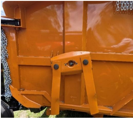
Oval stump jumping disc protects the carrier.
